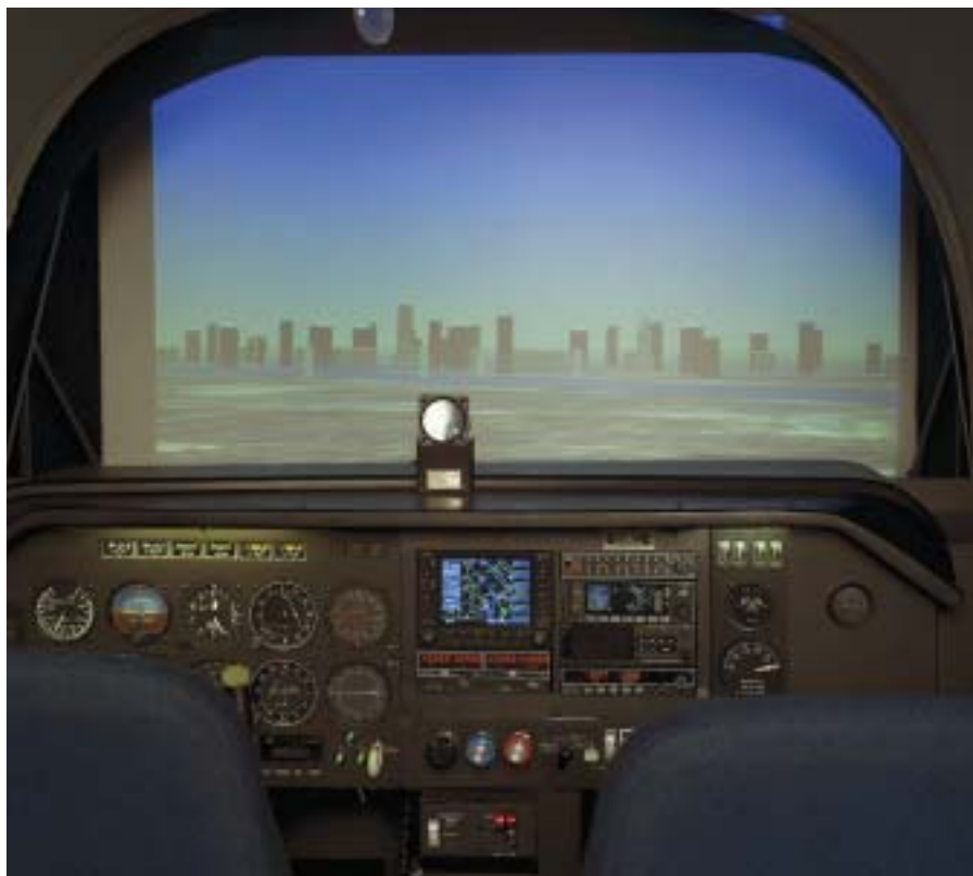
Flight Level Aviation’s flight training device is a hybrid—a traditional FTD on a motion base. Visual displays increase realism for training scenarios.
