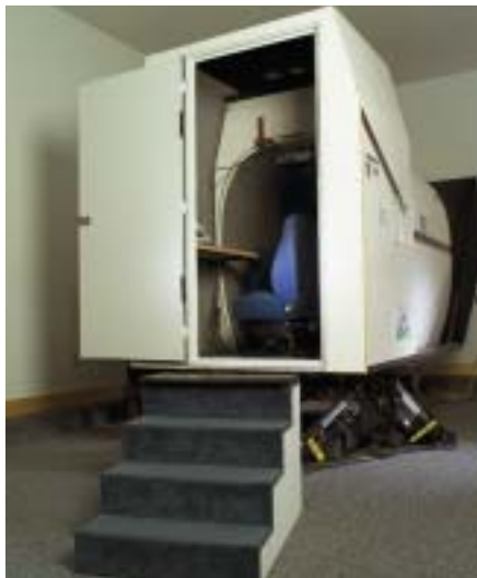
The motion base simulates turbulence and other aircraft flight characteristics.
